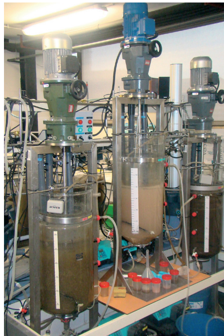
Planta pilot Granular-SBR Granular-SBR pilot plant
