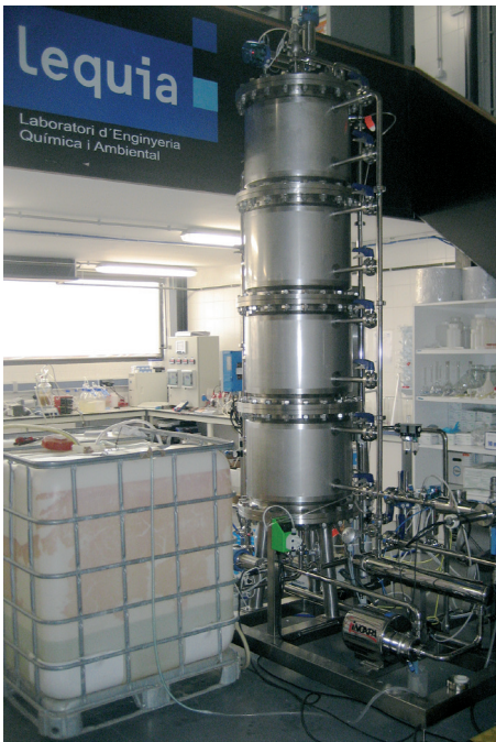
Planta pilot anammox Anammox pilot plant
