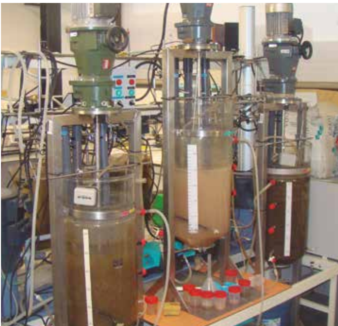
SBR pilot plant ↗
