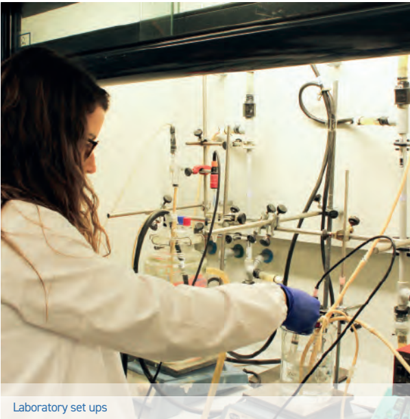
Hydrogen measurements in a bioelectrochemical system
